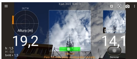
Fig. 7. eNodeB1 Height Measurement with Smart Measure.
