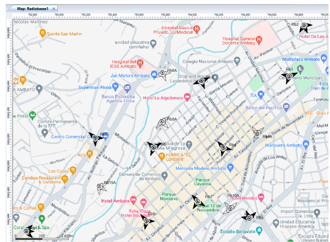
Fig. 8. Distribution of the base station transmitters in the simulation environment using professional planning software.
