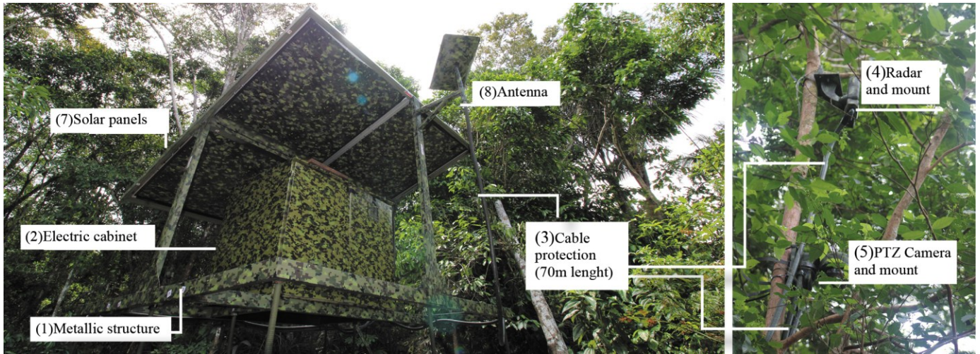
Fig. 4. Final RMS prototype installed in the Amacayacu National Natural Park (December 2024).
