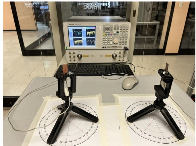
Fig. 5. Experimental setup showing the VNA and an antenna connected to each port.
