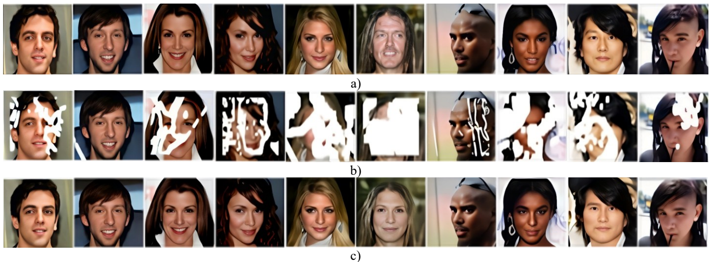
Fig. 7. a) Original image, I . b) Image with a binary mask, I_m . c) Image reconstructed by I_{\text{FACE}}\text{NET} .
