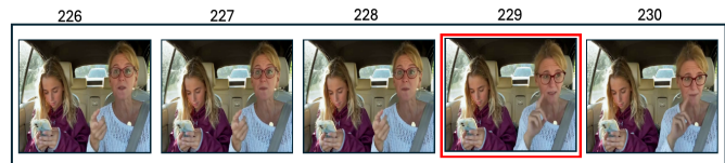
Fig. 3. The figure illustrates a sequence of frames extracted from the manipulated video “deleted KATIE GETS HER DRIVERS PERMIT!!_first time driving_4_2” from the DTD dataset. The frames are displayed chronologically, with their indices shown above each frame. A discontinuity in the temporal sequence is observed between the 228th and 229th frames, where 59 frames were omitted in the manipulated video. Consequently, the 229th frame has been marked as manipulated and is highlighted with a red border to emphasize this annotation.
