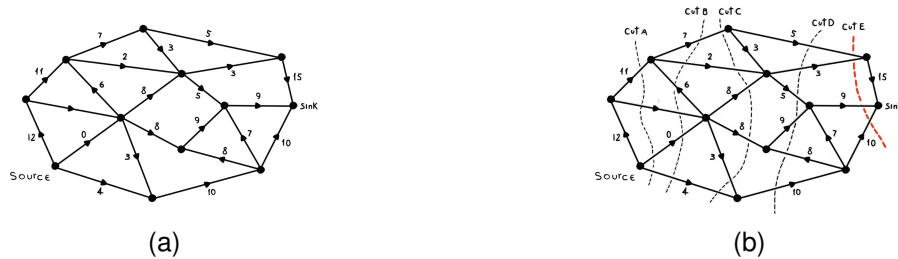
Fig. 1. Representation of a large-scale flow network, showing source(s), sink(t), and various possible slices. (a) source node and sink node. (b) graph cuts
