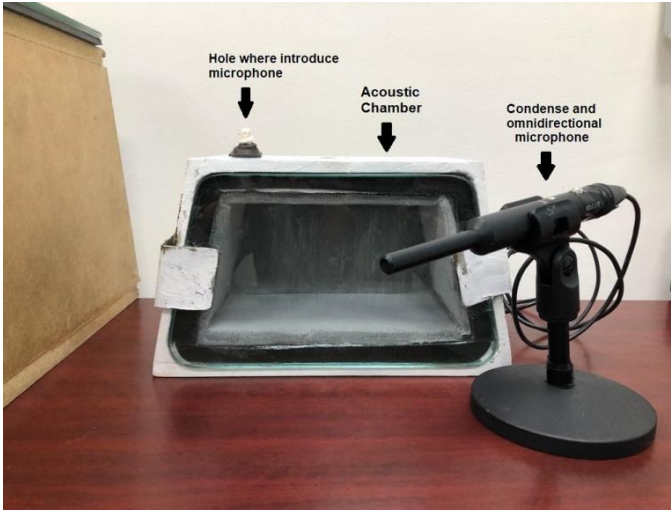
Fig. 4. Acoustic chamber used for recording of wingbeat signals.
