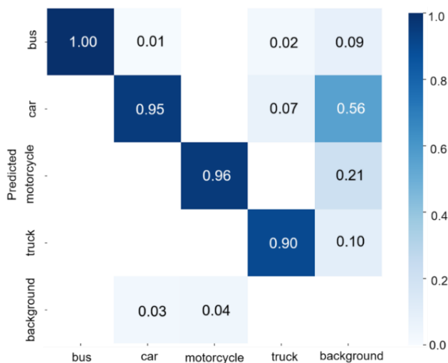
Fig. 7. Confusion matrix of YOLOv5 L with COCO-vehicle and specific dataset.
