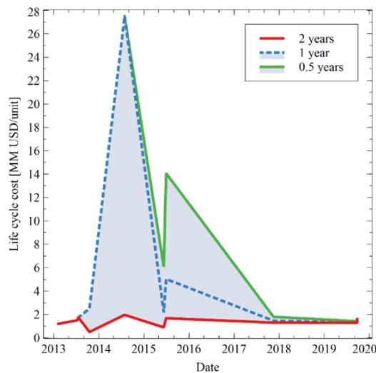
Fig. 12 Life cycle cost estimation for Spire cubesats.
