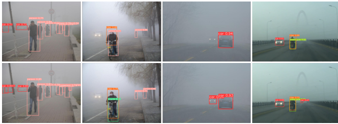
Fig. 5. Detection results of real foggy traffic image, the first and second rows are the results of the baseline YOLOv5 and the proposed model in this paper, respectively.
