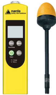
Fig. 2: Narda NBM-520 e sonda NBM E-Field-Probe EF0691 [23].
