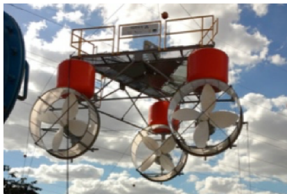
Fig. 10. Hydro-K turbine platform produced by the University of Brasilia with a nominal power of 30 kW.
