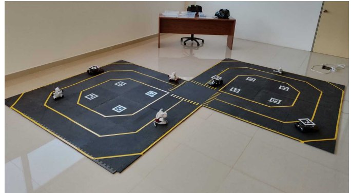
Fig. 1. DonkieTown , a low-cost scalable experimental platform for autonomous cars. Here, a lemniscate-like road is depicted, showing the Asinus Cars autonomously navigating while avoiding donkey-like obstacles.
