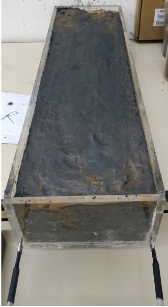
Fig. 5. Iron ore inserted in the prototype.
