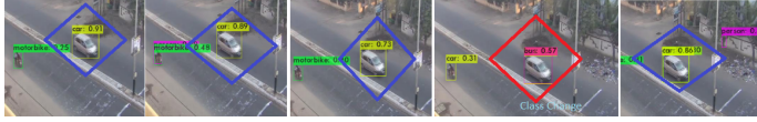
Fig. 3. Extracted Vehicle in consecutive frames with class change and drastic change in Confidence Score.
