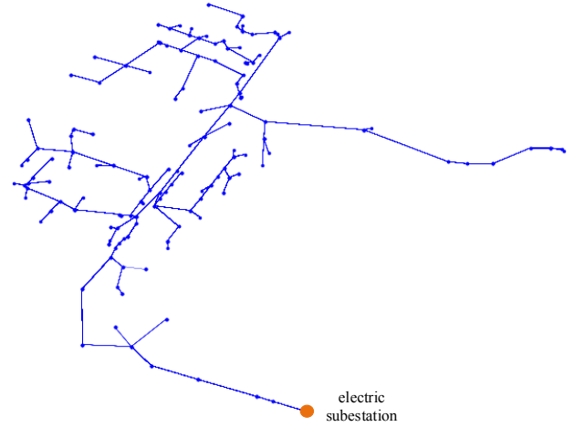
Fig. 11. Three-phase Mexican tested feeder.
