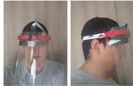
Fig. 2. Face shield HUD Prototype. This device contains the camera sensor and the workers' health monitoring sensors.
