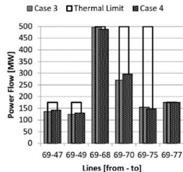
Fig. 6. Power flow and thermal limit in each line
