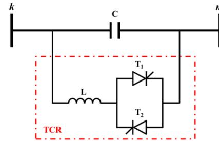
Fig. 1. Basic one-line diagram of TCSC.
