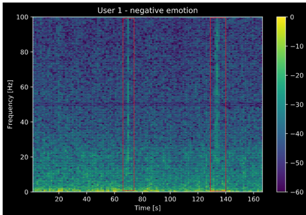
Fig. 5. Normalized spectrogram of the FT7 electrode with spectral density in dB of subject 1. In this trial, a negative emotion is stimulated.
