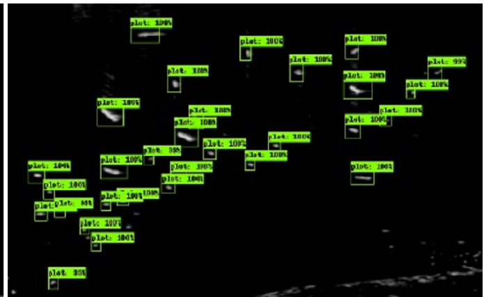
Fig. 6. Prediction results with the same set of hyperparameters in different training order: (a) Bounding box annotations in the 1st training with Recall=0.3333 and Loss function=0.5598; (b) Bounding box annotations in the 24th training with Recall=0.9091 and Loss function=0.0042.
