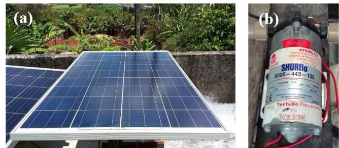
Fig. 4. (a) Panel fotovoltaico YL95; (b) Motor-bomba Shurflo 8000.
