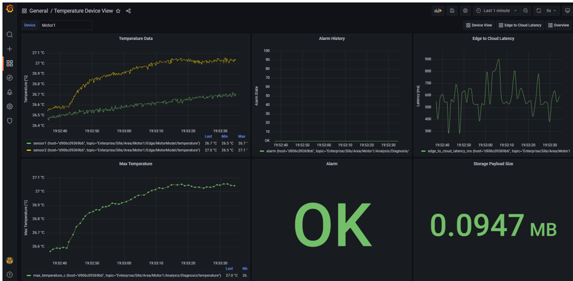
Fig. 9. Client view for the temperature monitoring case.
