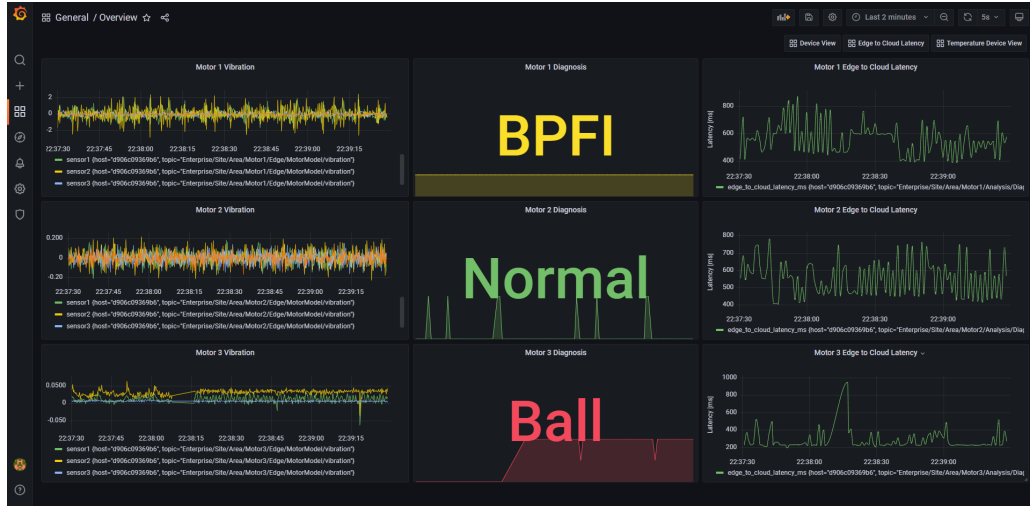
Fig. 5. Grafana dashboard monitoring three physically independent edge nodes concurrently.
