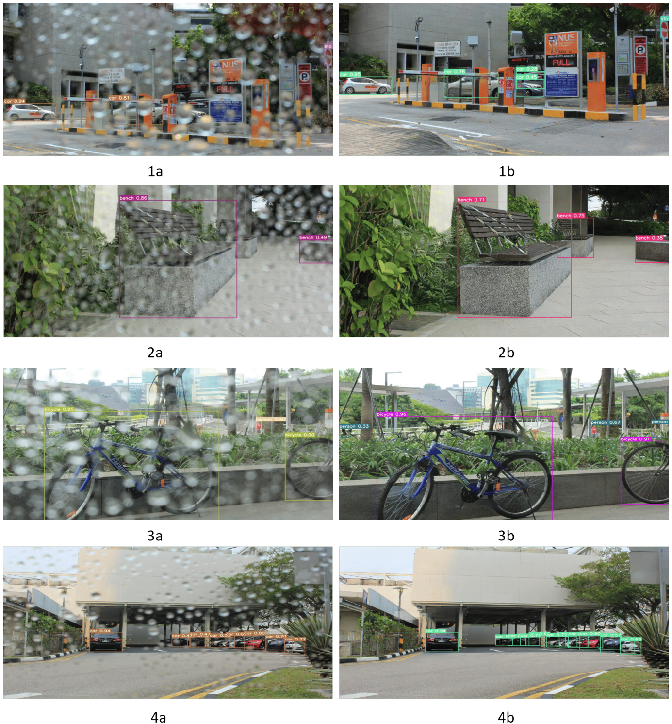
Fig. 4. Visual impact of D2W-GAN-based raindrop removal on object detection accuracy for test images 1–4. (a) Raindrop-degraded images with YOLOv7-d6 detections. (b) D2W-GAN-enhanced images with YOLOv7-d6 detections.
