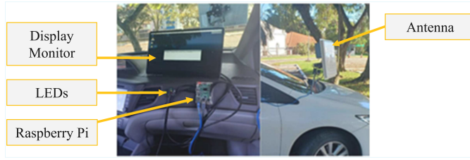
Fig. 5. Integration of the RFID perception subsystem on the test vehicle for field experiments. The forward-facing Viaonda MID 12-iETH antenna is mounted on a custom external support structure on the vehicle roof. The Raspberry Pi processing unit, LED status indicators, and an onboard display monitor are installed inside the cabin solely for monitoring purposes; none of these components influenced the recognition results.
