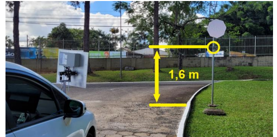
Fig. 4. RFID tag installation on the supporting pole of a traffic sign on the UniSATC campus at a standardized mounting height of 1.6 m ( \pm 20 cm). Tags are encapsulated in ABS material with IP68 rating, designed for metallic surface installation compatible with standard sign poles. This mounting height was maintained consistently across all 12 field-test signs.
