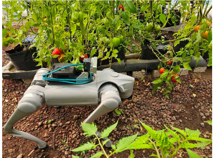
Fig. 1. Testing scene. The robot detects the ripening stage of the tomatoes in a real scenario. Even though the available dataset was captured in laboratory, our proposed method generates datasets that can be used for training a model that can detect tomatoes in the real scene.
