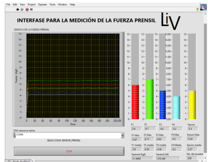
Fig. 6. Front panel of the graphical interface developed in LabVIEW for measuring the grip force of four fingers (F1–index, F2–middle, F3–ring, and F4–little).
