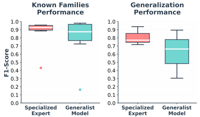
Fig. 3. F1-score distribution comparison between specialized wordlist expert and generalist model trained on 54 DGA families. Left: performance on known families (specialist 86.7% vs generalist 79.2%). Right: generalization to unknown families (specialist 80.9% vs generalist 62.1%). Box plots show median, quartiles, and outliers. Both models use identical ModernBERT architecture.
